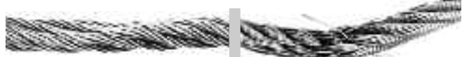
Crushing. Because of loose winding on drum, rope was pulled in between underlying wraps and crushed out of shape.
