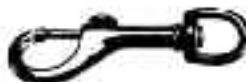
no. 225X Swivel eye Snaps cast malleable iron nickel plated Long body – snap takes 5/8 rope
